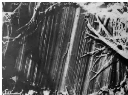
Figure 5. Electron micrograph of a fracture surface of polyethylene crystallized under 4800 atm pressure at 226°C. Scale 0.5 \mu\text{m} .
